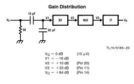
The IF gain could also be varied by changing the value of R6 across the IF output coil. However, it is a good idea to maintain a high Q IF tank in order to achieve good adjacent channel rejection. In order to prevent distortion due to overloading the IF amplifier, it is important that the impedance Pin 14 sees looking into the IF output tank, T5, does not go below 3K ohms.
