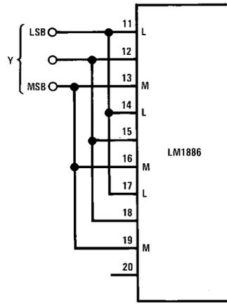
FIGURE 2b. 8-level Grey Scale Input Connection
