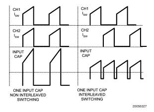
FIGURE 12. Switch and Input Capacitor Currents
