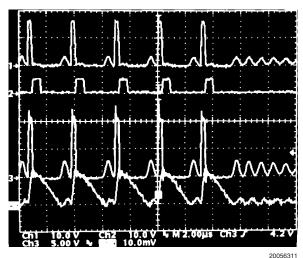
20056; CH1: HDRV, CH2: LDRV, CH3: SW, CH4: I<sub>1</sub> (0.2A/div)
