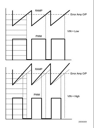
FIGURE 1. Voltage Feedforward
