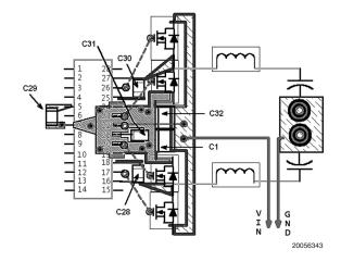
FIGURE 14. Critical Component placement (TSSOP)
