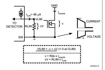
FIGURE 11. Understanding Current Sensing
