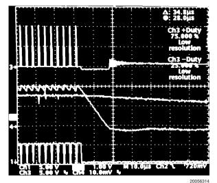
CH1: LDRV, CH2: Vo, CH3: SW, CH4:  $I_L$  (1A/div) Output 1V @ 2A, VIN = 10V, FPWM/SKIP, L = 10 $\mu$ H, f = 300kHz,  $C_{QUT}$  =
