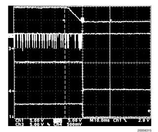
CH1: PGOOD, CH2: VIN, CH3: LDRV, CH4: Vo Output 1V @ 0.02A, VIN = 9.75V, FPWM, L =  $10\mu$ H, f = 300kHz,  $C_{OUT}$  =
