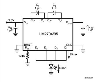
FIGURE 5. One Parallel Connected LED
