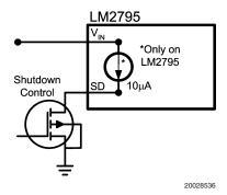
FIGURE 1. Open-Drain Logic Shutdown Control
