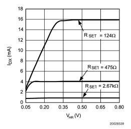
FIGURE 3.  $I_{LED}$  vs  $V_{HR}$ 4 LEDs,  $V_{IN} = 3.0V$
