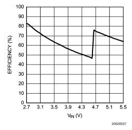
FIGURE 6. Efficiency vs  $V_{IN}$  4 LEDs,  $V_{LED} = 3.6V$ ,  $I_{LED} = 15mA$
