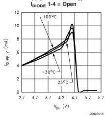
Shutdown Threshold vs V<sub>IN</sub>
