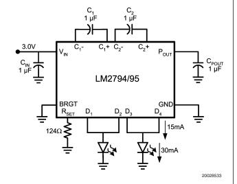
FIGURE 4. Two Parallel Connected LEDs
