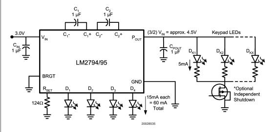
FIGURE 2. Keypad LEDs Connected to  $P_{\text{OUT}}$
