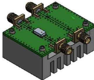
The evaluation board is supplied mounted on a heat sink. The maximum RF input power specified in the absolute maximum ratings table must not be exceeded.
