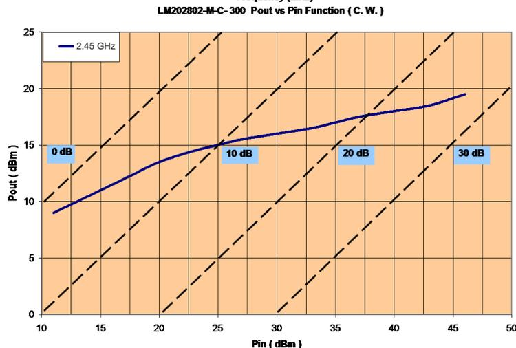
Output Power vs. Input Power,  $f = 2.45 \text{ GHz}$
