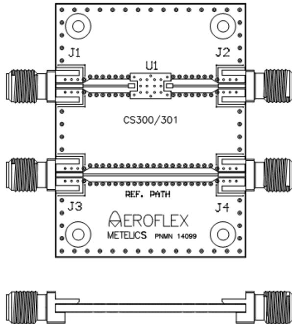
The evaluation board for the LM202802-M-C-300 is shown above. This evaluation board comprises two sections: the evaluation circuit for the LM202802-M-C-300 limiter module (U1); and, a reference path transmission line.
