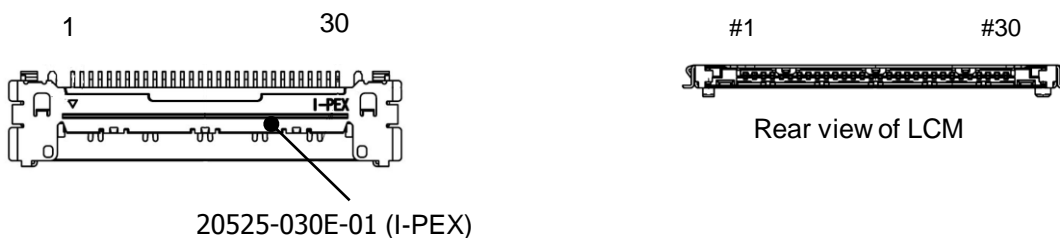
[ Figure 3 ] User Connector diagram
