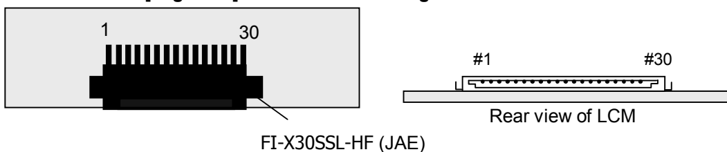
[ Figure 4 ] User Connector diagram
