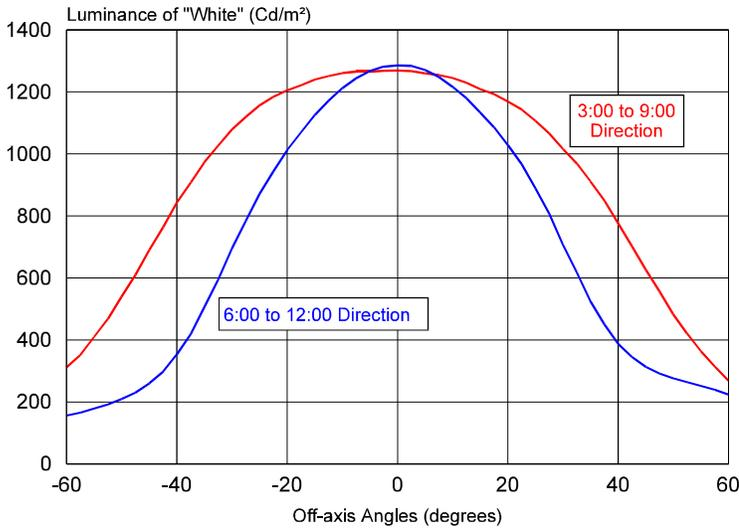
At the optimal viewing directions, the LM222-170EG01 LCD module has a very high contrast ratio (CR) of about 1,000:1. This is the inherent CR, which is the luminance ratio between the “White” and the “Black” states measured in a dark room. Under ambient lighting, particularly in bright outdoor environments, the CR value of the display drops significantly due to the reflection and glare caused by the strong ambient illumination.
