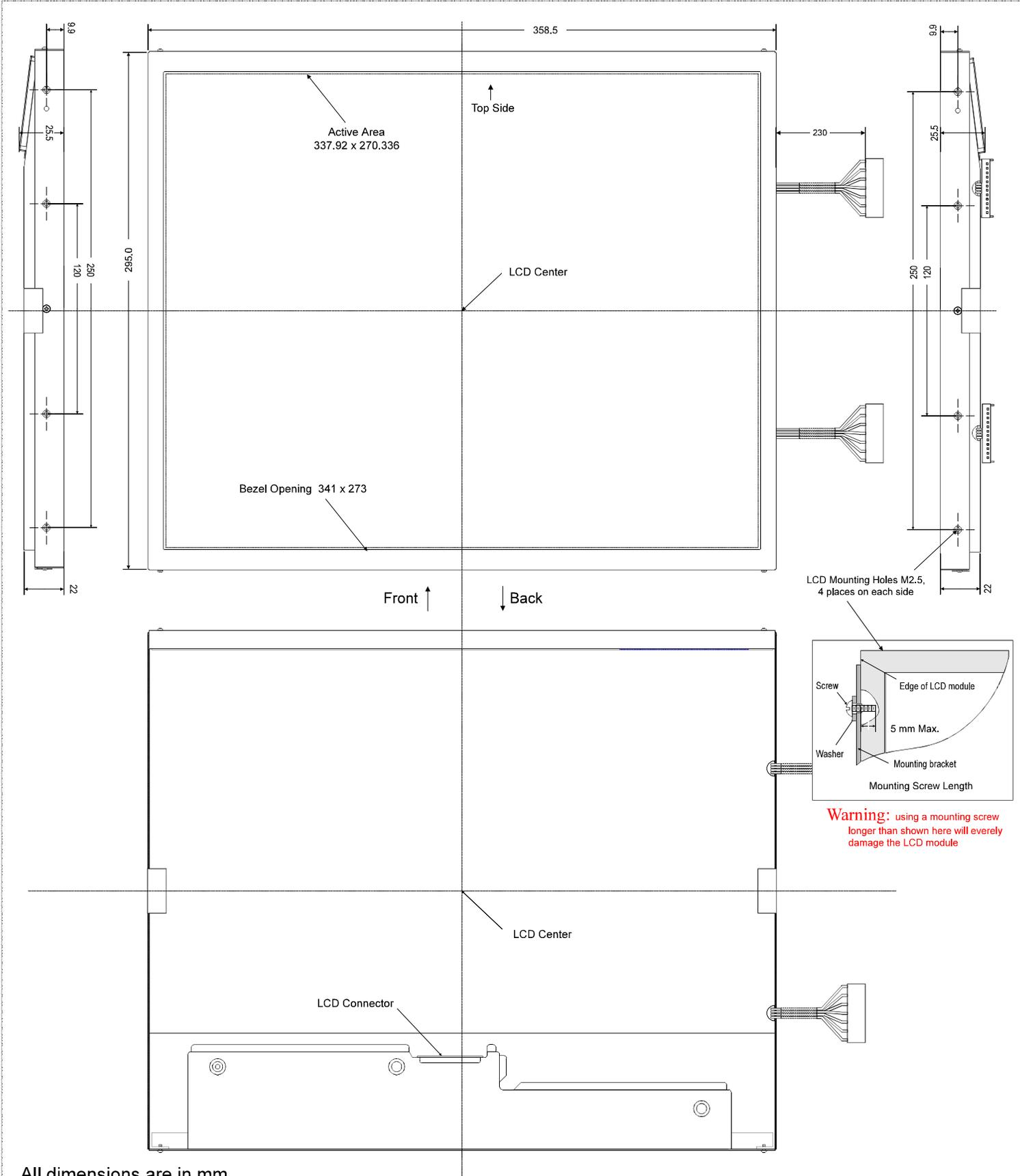
**Warning:** using a mounting screw longer than shown here will everely damage the LCD module
