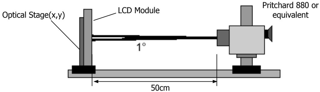
**FIG. 1 Optical Characteristic Measurement Equipment and Method**
