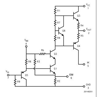
FIGURE 2. Simplified Schematic Diagram
