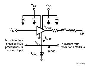
FIGURE 14. Simplified IK Interface for Current Feedback Systems
