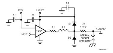
FIGURE 12. Recommended Application Circuit
