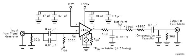
Note: 10pF load includes parasitic capacitance.
