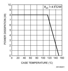
FIGURE 10. Power Derating Curve
