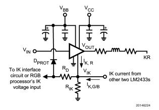
FIGURE 13. Simplified IK Interface for Voltage Feedback Systems
