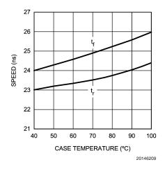
FIGURE 8. Speed vs Case Temperature
