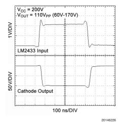
FIGURE 11. Cathode Pulse Response
