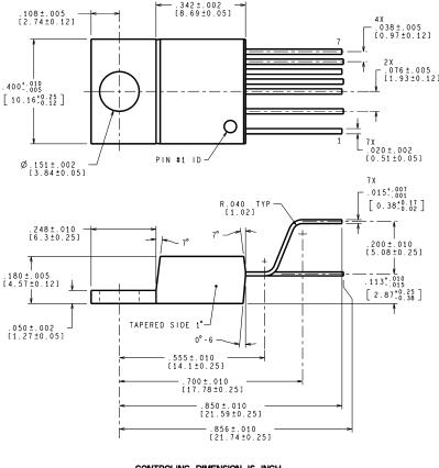
CONTROLING DIMENSION IS INCH VALUES IN [ ] ARE MILLIMETERS
