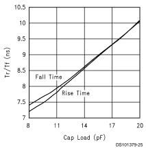
FIGURE 10. Speed vs. Load
