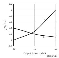
FIGURE 9. CRT Driver Speed vs. Offset
