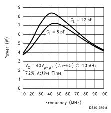
FIGURE 8. CRT Driver Power Dissipation vs. Frequency
