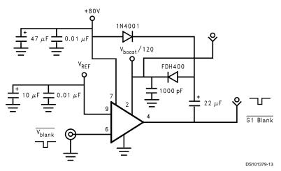
FIGURE 13. 120V Boost/G1 Drive Test Circuit
