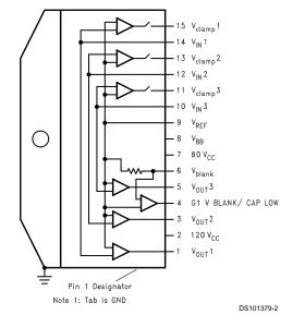
FIGURE 2. LM2457 Package Pinout Order Number LM2457TA
