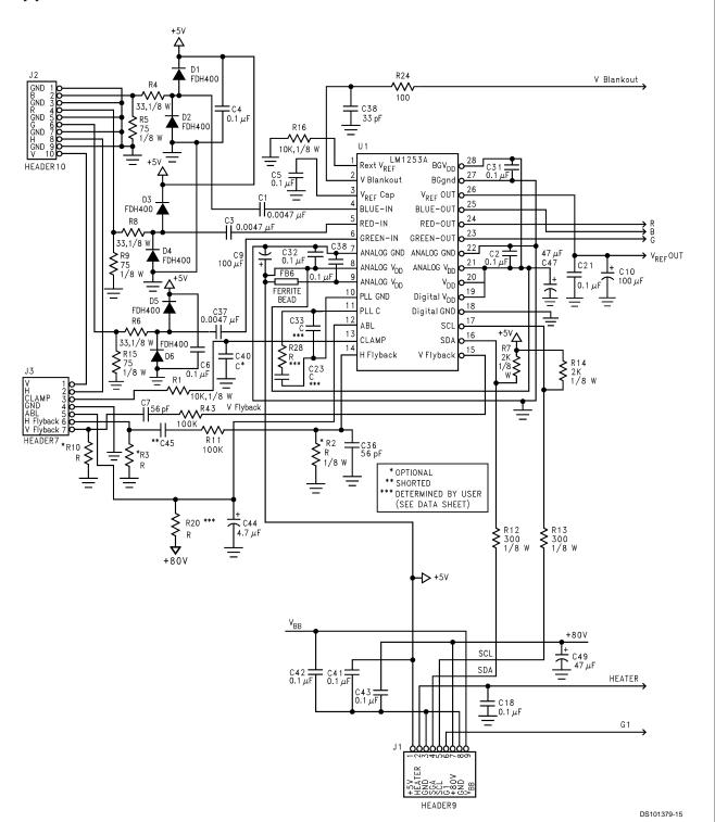
FIGURE 17. LM1253A/245X Reference Design Schematic
