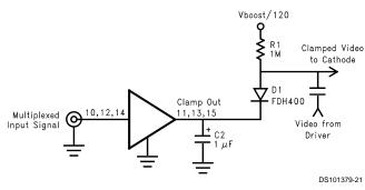
FIGURE 15. Clamp Application Circuit.
