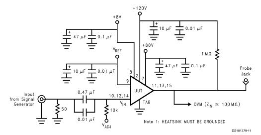
FIGURE 11. Test Circuit (One Channel)
