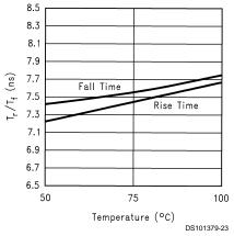
FIGURE 6. CRT Driver Speed vs. Temperature
