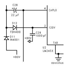
FIGURE 16. Boost Circuit Schematic
