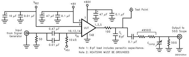
FIGURE 4. Test Circuit (One Channel)
