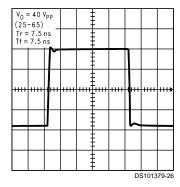
FIGURE 7. CRT Driver Transient Response
