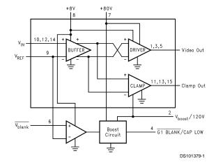
FIGURE 1. LM2457 Block Diagram
