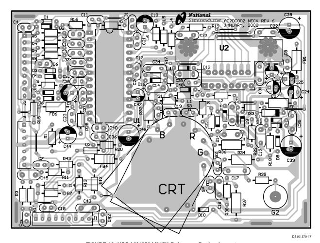
FIGURE 19. NSC LM1253A/245X Reference Design Layout
