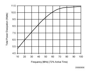
FIGURE 6. Power Dissipation vs Frequency
