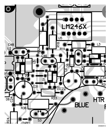
FIGURE 13. Trace Routing and Component Placement for Blue Channel Output
