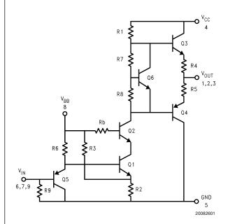
FIGURE 1. Simplified Schematic Diagram (One Channel)
