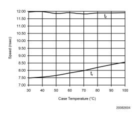
FIGURE 4. Speed vs Case Temperature
