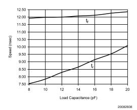
FIGURE 8. Speed vs Load Capacitance
