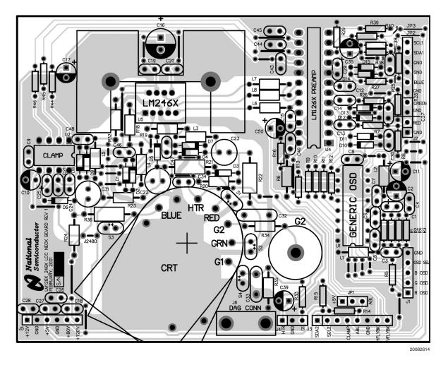
FIGURE 12. LM126X/246X Demo Board Layout
