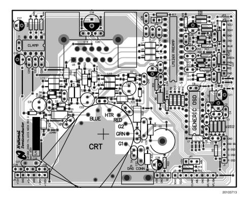
FIGURE 12. NSC Demonstration Board Layout
