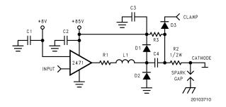
FIGURE 9. One Channel of the LM2471 with the Recommended Application Circuit
