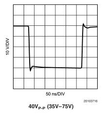
FIGURE 10. Typical Cathode Response
