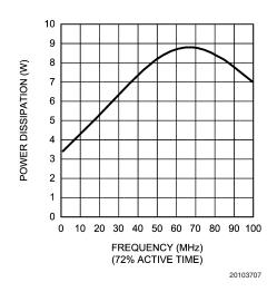
FIGURE 6. Power Dissipation vs Frequency
