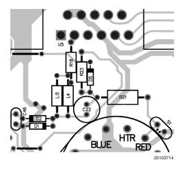
FIGURE 13. Trace Routing and Component Placement for Red Channel Output
