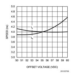
FIGURE 7. Speed vs Offset
