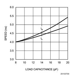
FIGURE 8. Speed vs Load Capacitance
