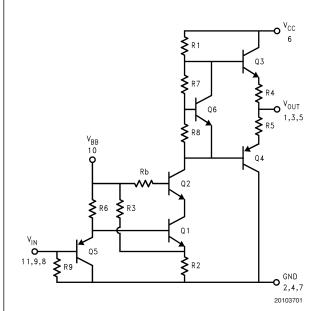
FIGURE 1. Simplified Schematic Diagram (One Channel)
