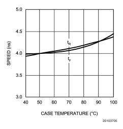
FIGURE 4. Speed vs Temp.
