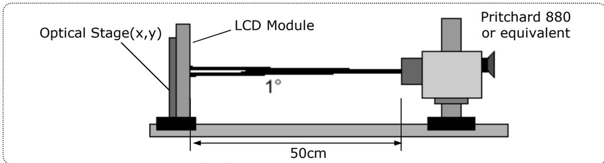
**FIG. 4 Optical Characteristic Measurement Equipment and Method**
