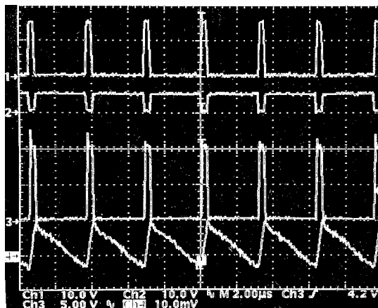
Figure 4. Normal FPWM Mode Operation at Light Loads
