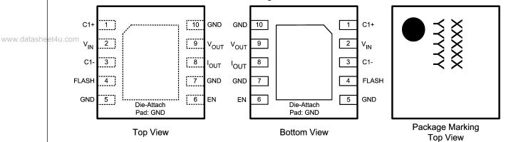
**Note**: The actual physical placement of the package marking will vary from part to part. The package marking placeholder "XXXXX" is a code for die traceability. "YYYYY" identifies the device (part number, voltage option, etc.). See the Order Information table below for the device ID codes.
