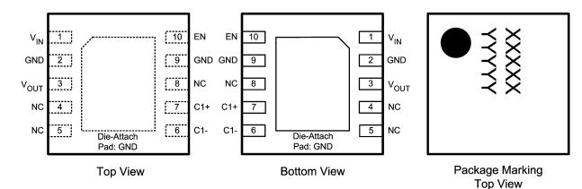
**Note**: The actual physical placement of the package marking will vary from part to part. The package marking placeholder "XXXXX" is a code for die traceability. "YYYYY" identifies the device (part number, voltage option, etc.). See the Order Information table below for the device ID codes.
