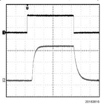
CH1:  $V_{EN}$ ; Scale: 2V/Div, DC Coupled CH2:  $V_{OUT}$ ; Scale: 500mV/Div, DC Coupled
