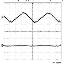
CH1:  $V_{IN}$ ,  $C_{IN}=1\mu F$ ; Scale: 50mV/Div, AC Coupled CH2:  $V_{IN}$ ,  $C_{IN}=10\mu F$ ; Scale: 50mV/Div, AC Coupled Time scale: 200ns/Div
