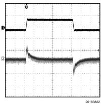
CH1: V<sub>IN</sub>; Scale: 1V/Div, AC Coupled CH2:  $V_{OUT}$ ; Scale: 20mV/Div, AC Coupled
