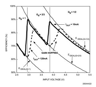
FIGURE 1. Efficiency of LM2788-1.8 with 10mA and 120mA output currents Base-gain ( $G_B$ ) regions are separated and labeled Ideal efficiency curves of charge pumps with G =1/2, 2/3, and 1 are included ( $E_{IDEAL(G=1)}$ ,  $E_{IDEAL(G=2/3)}$ ,  $E_{IDEAL(G=1/2)}$ )
