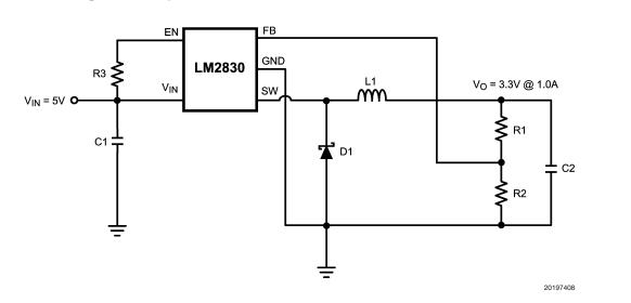
FIGURE 8. LM2830X (1.6MHz): Vin = 5V, Vo = 3.3V @ 1.0A
