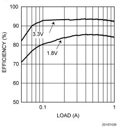
$\eta$  vs Load "X and Z" Vin = 3.3V, Vo = 1.8V
