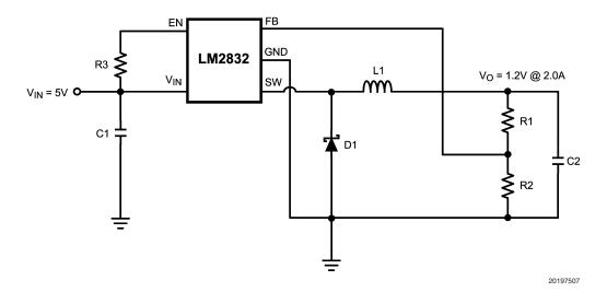
FIGURE 6. LM2832X (1.6MHz): Vin = 5V, Vo = 1.2V @ 2.0A
