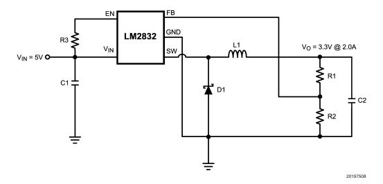
FIGURE 8. LM2832X (1.6MHz): Vin = 5V, Vo = 3.3V @ 2.0A
