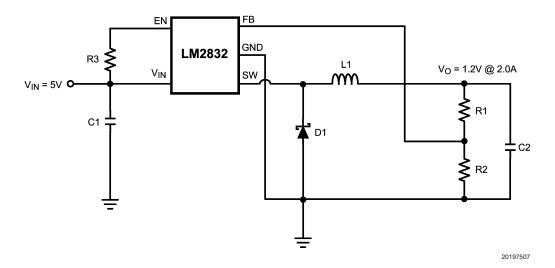
FIGURE 12. LM2832Z (3MHz): Vin = 5V, Vo = 1.2V @ 2.0A
