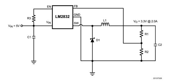
FIGURE 11. LM2832Z (3MHz): Vin = 5V, Vo = 3.3V @ 2.0A
