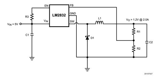
FIGURE 10. LM2832Y (550kHz): Vin = 5V, Vout = 1.2V @ 2.0A
