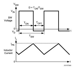
FIGURE 2. Typical Waveforms
