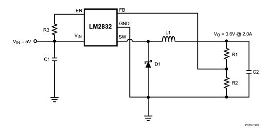
FIGURE 7. LM2832X (1.6MHz): Vin = 5V, Vo = 0.6V @ 2.0A
