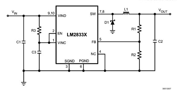
FIGURE 11. LM2833X (1.5MHz):  $V_{IN} = 3.3V$ , Output = 1.2V/3.0A
