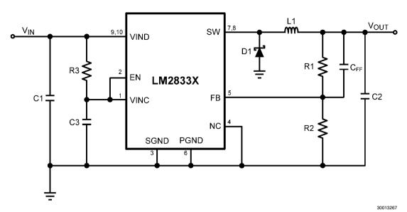
FIGURE 12. LM2833X (1.5MHz):  $V_{IN} = 5V$ , Output = 3.3V/3.0A
