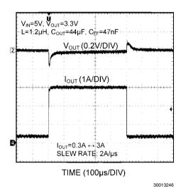
FIGURE 10. Load Step Response with CFF
