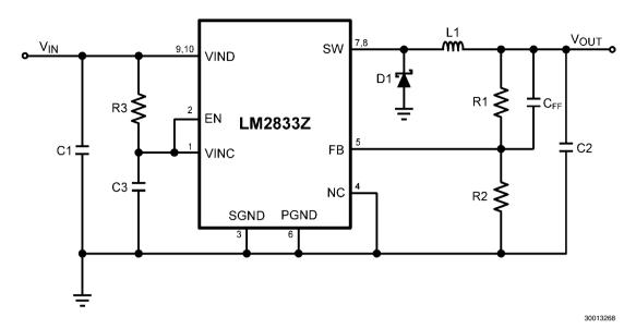
FIGURE 14. LM2833Z (3MHz):  $V_{IN} = 5V$ , Output = 3.3V/3.0A
