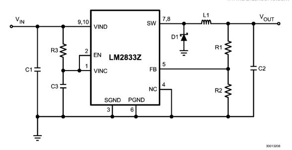
FIGURE 13. LM2833Z (3MHz):  $V_{IN} = 3.3V$ , Output = 1.2V/3.0A
