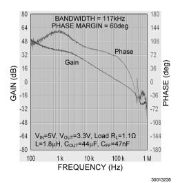
FIGURE 8. Loop Gain and Phase with C<sub>FF</sub>
