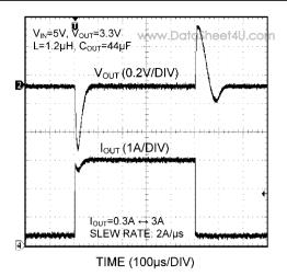
FIGURE 9. Load Step Response without C<sub>FF</sub>
