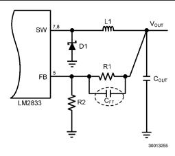
FIGURE 6. Adding a C<sub>FF</sub> Capacitor
