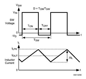
FIGURE 2. SW Pin Voltage and Inductor Current Waveforms
