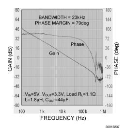
FIGURE 7. Loop Gain and Phase without CFF
