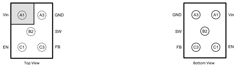
Figure 3. 5 Bump DSBGA YZR and YPD Package (YPD package to be released soon)
