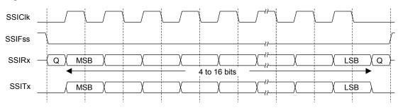
Figure 12-6. Freescale SPI Frame Format with SPO=0 and SPH=1
