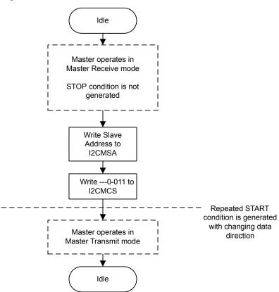
Figure 13-12. Master Burst SEND after Burst RECEIVE
