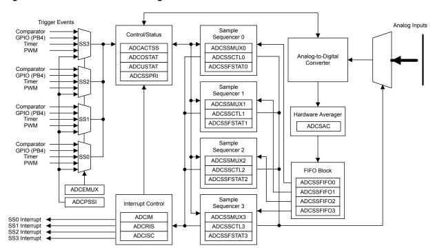
Figure 10-1. ADC Module Block Diagram
