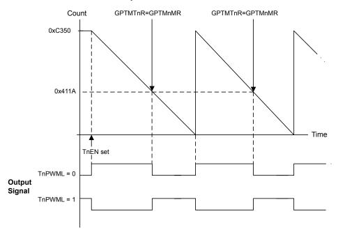
Figure 8-4. 16-Bit PWM Mode Example
