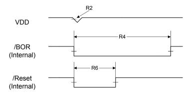
Figure 17-8. Software Reset Timing
