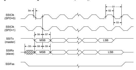
Figure 17-14. SSI Timing for SPI Frame Format (FRF=00), with SPH=1
