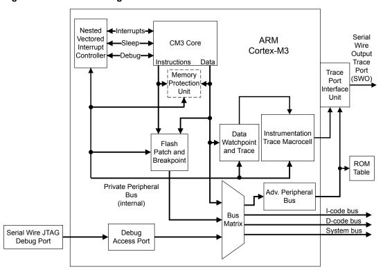
Figure 2-1. CPU Block Diagram
