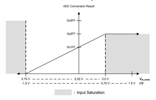
Figure 10-4. Differential Sampling Range,  $V_{IN\ ODD}$  = 2.25 V
