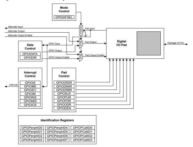
Figure 7-2. GPIO Port Block Diagram
