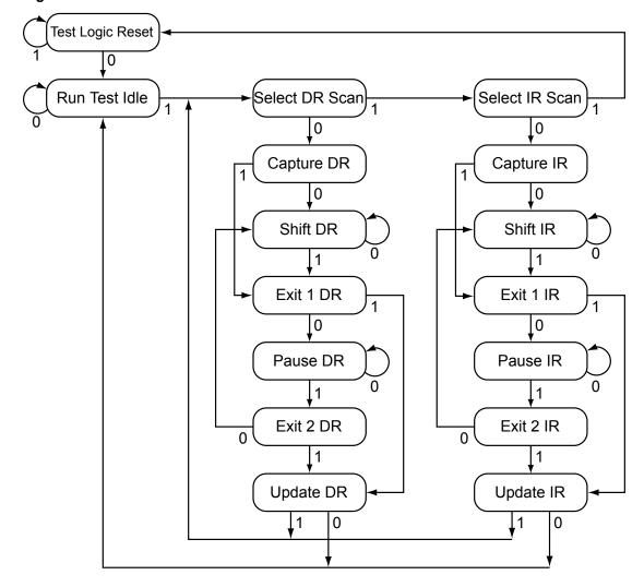
Figure 4-2. Test Access Port State Machine
