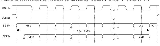
Figure 12-7. Freescale SPI Frame Format (Single Transfer) with SPO=1 and SPH=0
