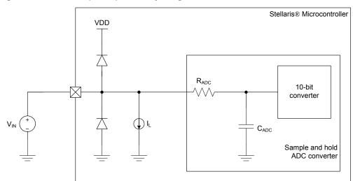
Figure 17-11. ADC Input Equivalency Diagram
