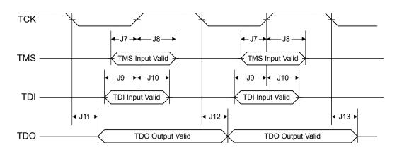
Figure 17-3. JTAG Test Access Port (TAP) Timing
