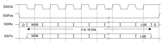
Figure 12-9. Freescale SPI Frame Format with SPO=1 and SPH=1
