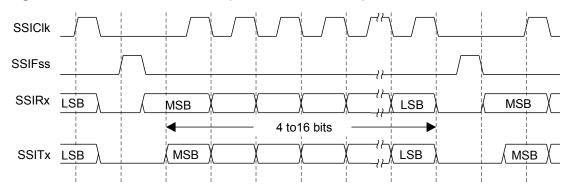
Figure 12-5. Freescale SPI Format (Continuous Transfer) with SPO=0 and SPH=0
