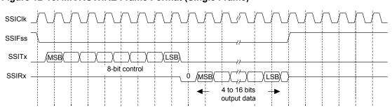
Figure 12-10. MICROWIRE Frame Format (Single Frame)
