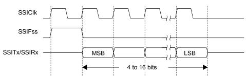
Figure 12-2. TI Synchronous Serial Frame Format (Single Transfer)
