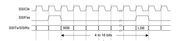
Figure 12-3. TI Synchronous Serial Frame Format (Continuous Transfer)
