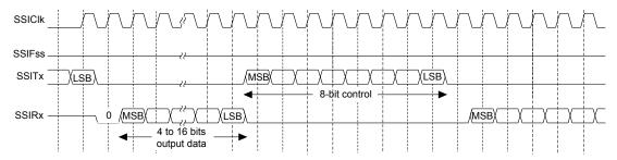
Figure 12-11. MICROWIRE Frame Format (Continuous Transfer)
