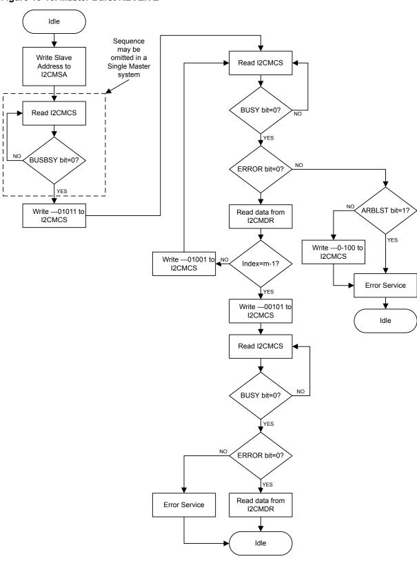
Figure 13-10. Master Burst RECEIVE
