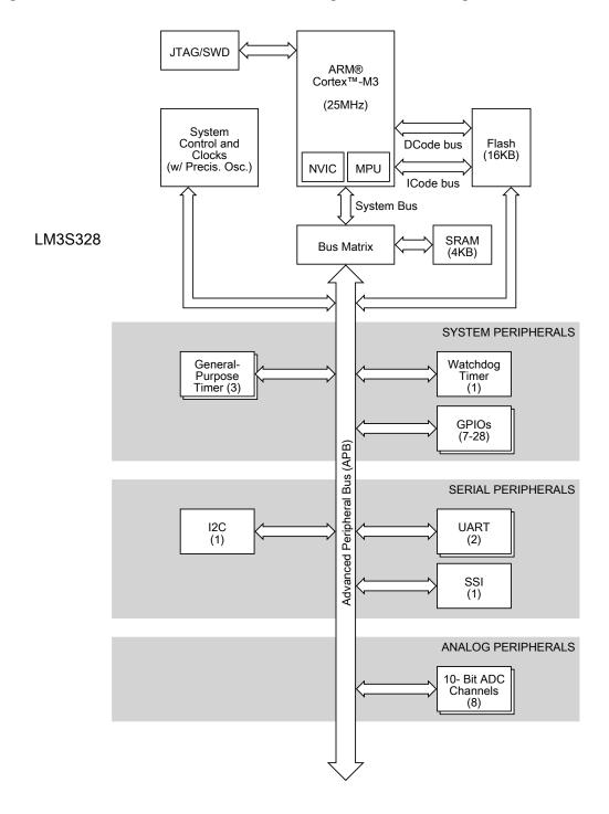
Figure 1-1. Stellaris LM3S328 Microcontroller High-Level Block Diagram
