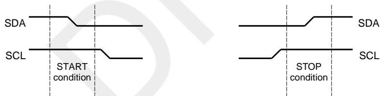
Figure 14-3. START and STOP Conditions
