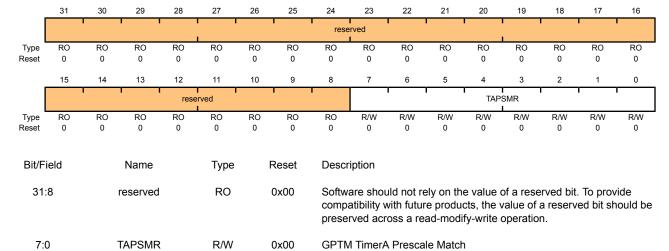
This value is used alongside **GPTMTAMATCHR** to detect timer match events while using a prescaler.
