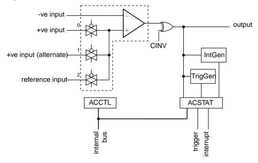
A comparator is configured through two status/control registers (ACCTL and ACSTAT). The internal reference is configured through one control register (ACREFCTL). Interrupt status and control is configured through three registers (ACMIS, ACRIS, and ACINTEN). The operating modes of the comparators are shown in the Comparator Operating Mode tables.
