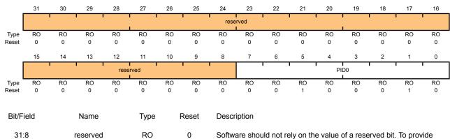
Can be used by software to identify the presence of this peripheral.
