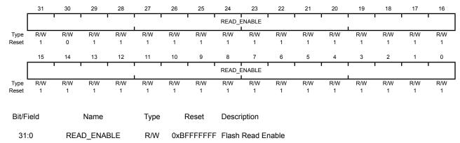
Each bit position maps 2 Kbytes of Flash to be read-enabled.
