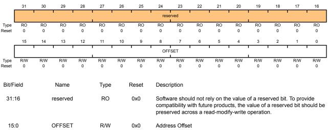
Address offset in flash where operation is performed.
