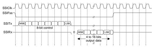
Figure 13-10. MICROWIRE Frame Format (Single Frame)
