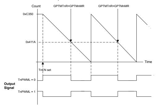
Figure 9-4. 16-Bit PWM Mode Example
