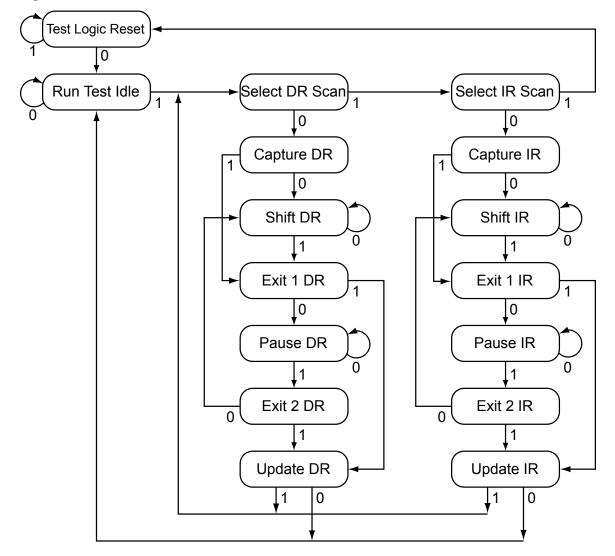
Figure 5-2. Test Access Port State Machine
