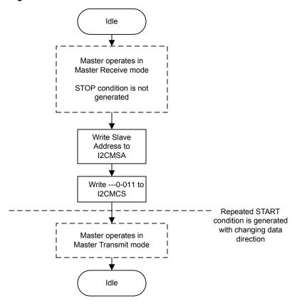
Figure 14-12. Master Burst SEND after Burst RECEIVE
