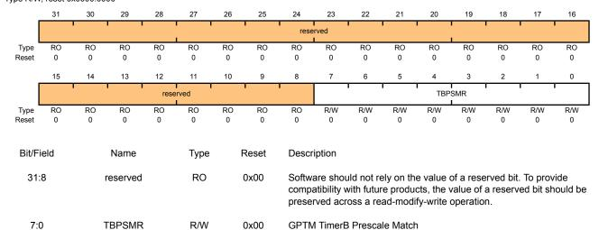
This value is used alongside **GPTMTBMATCHR** to detect timer match events while using a prescaler.
