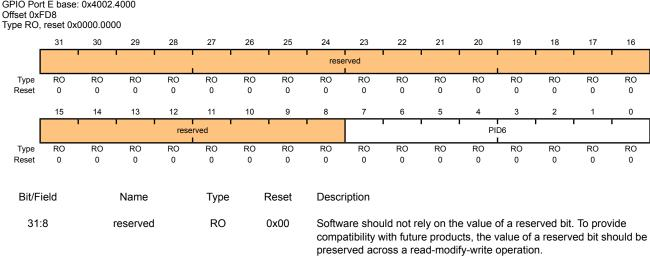
GPIO Peripheral ID Register[23:16]
