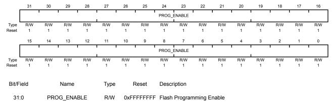
Each bit position maps 2 Kbytes of Flash to be write-enabled.
