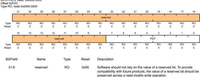
GPIO Peripheral ID Register[31:24]
