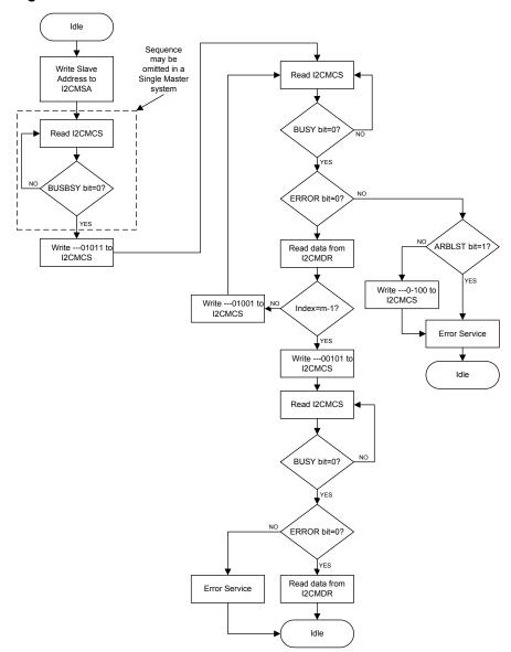
Figure 14-10. Master Burst RECEIVE
