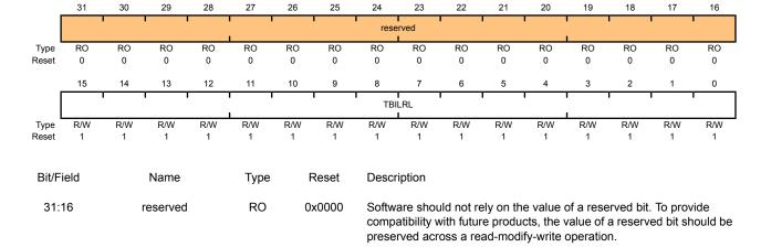
When the GPTM is not configured as a 32-bit timer, a write to this field updates **GPTMTBILR**. In 32-bit mode, writes are ignored, and reads return the current value of **GPTMTBILR**.
