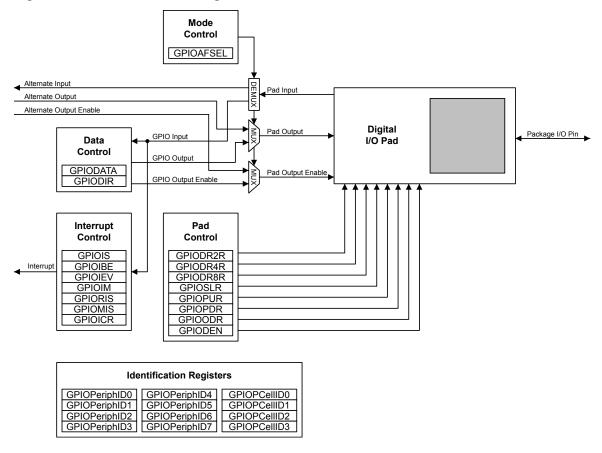
Figure 8-1. GPIO Port Block Diagram
