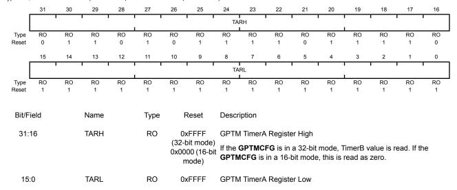
A read returns the current value of the **GPTM TimerA Count Register**, except in Input Edge Count mode, when it returns the timestamp from the last edge event.
