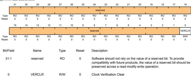
Clears clock verification faults.
