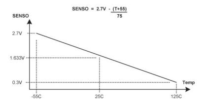
Figure 11-2. Internal Temperature Sensor Characteristic
