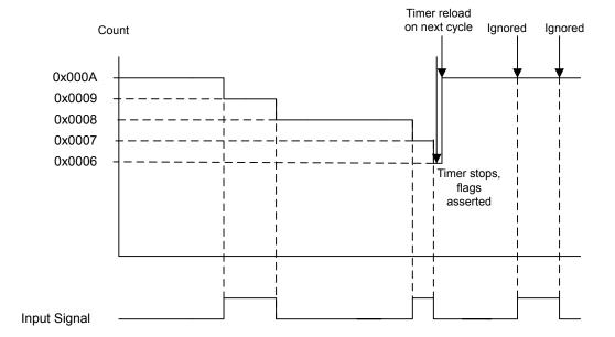
Figure 9-2. 16-Bit Input Edge Count Mode Example
