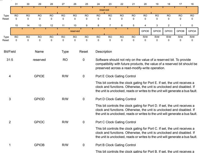
clock and functions. Otherwise, the unit is unclocked and disabled. If the unit is unclocked, reads or writes to the unit will generate a bus fault.
