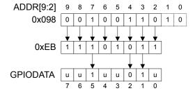
During a read, if the address bit associated with the data bit is set to 1, the value is read. If the address bit associated with the data bit is set to 0, it is read as a zero, regardless of its actual value. For example, reading address GPIODATA + 0x0C4 yields as shown in Figure 8-3 on page 126.
