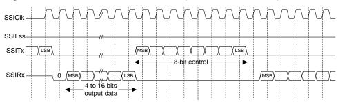
Figure 13-11. MICROWIRE Frame Format (Continuous Transfer)
