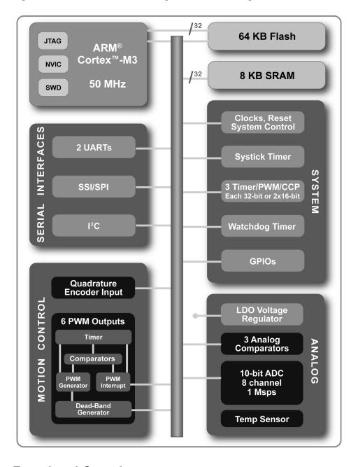
Figure 1-1. Stellaris<sup>®</sup> 800 Series High-Level Block Diagram
