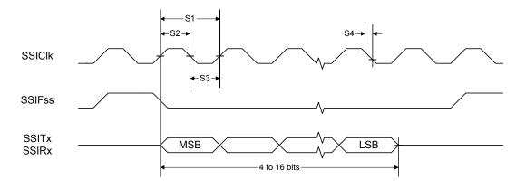
Figure 19-4. SSI Timing for MICROWIRE Frame Format (FRF=10), Single Transfer
