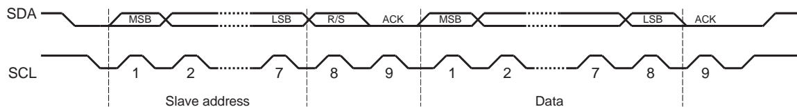
Figure 14-5. Complete Data Transfer with a 7-Bit Address
