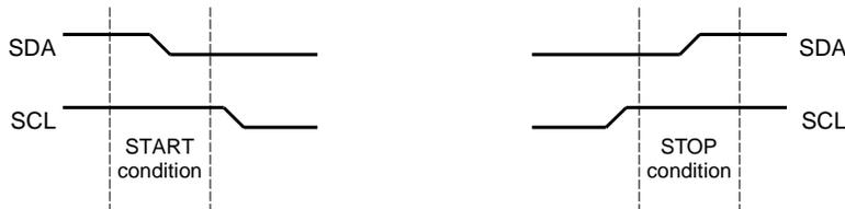
When operating in slave mode, two bits in the **I2CSRIS** register indicate detection of start and stop conditions on the bus; while two bits in the **I2CSMIS** register allow start and stop conditions to be promoted to controller interrupts (when interrupts are enabled).
