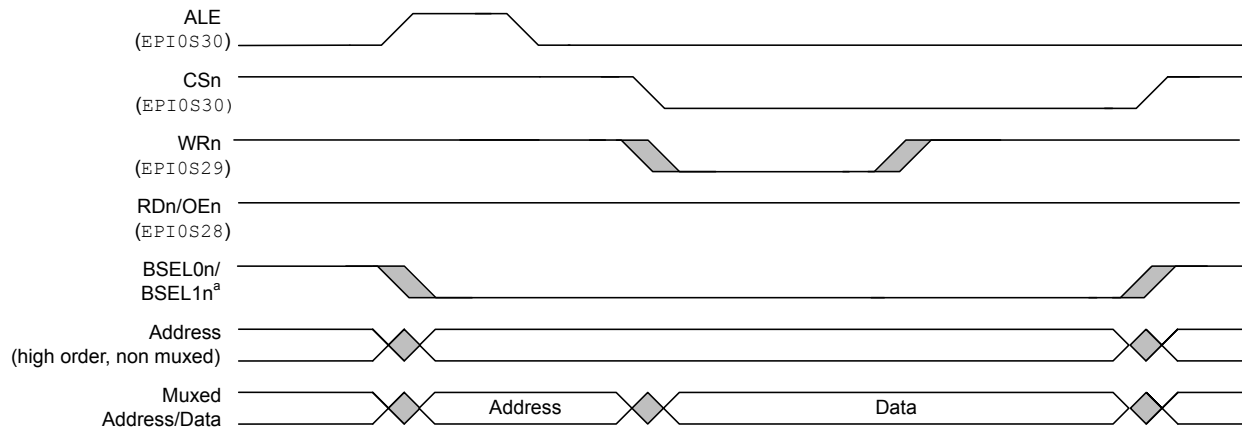
Figure 10-7. Host-Bus Write Cycle with Multiplexed Address and Data, MODE = 0x0, WRHIGH = 1, RDHIGH = 1
