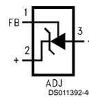
\*This pin must be left floating or connected to pin 2.
