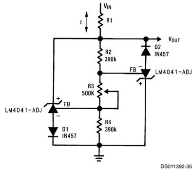
FIGURE 8. Bidirectional Adjustable
