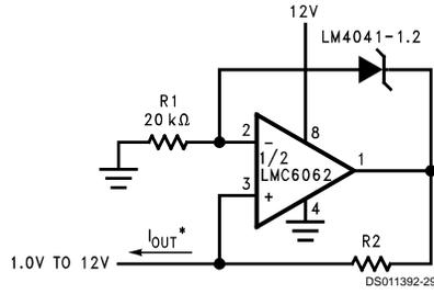
FIGURE 13. Precision 1 μA to 1 mA Current Sources
