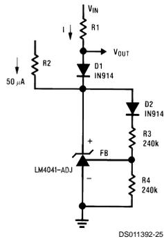
FIGURE 6. Fast Positive Clamp
