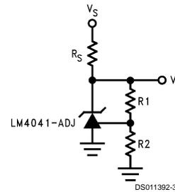
$$V_O = V_{REF}[(R_2/R_1) + 1]$$
