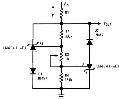
FIGURE 9. Bidirectional Adjustable
