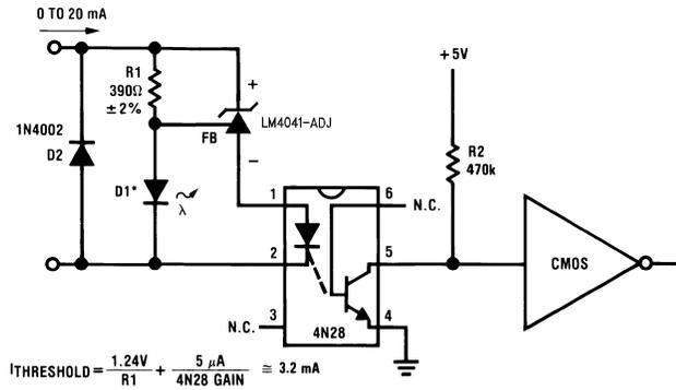
$$I_{\text{THRESHOLD}} = \frac{1.24\text{V}}{R_1} + \frac{5\ \mu\text{A}}{4\text{N}28\ \text{GAIN}} \cong 3.2\ \text{mA}$$
