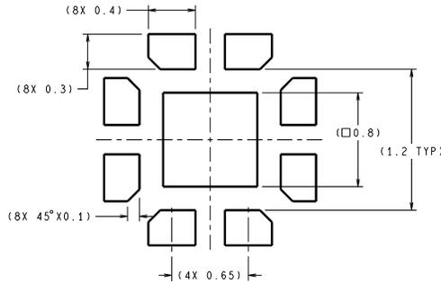
DIMENSIONS ARE IN MILLIMETERS
