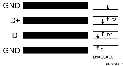
FIGURE 10. Ideal Diode Trace Layout
