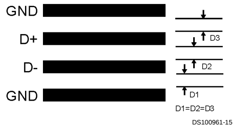
FIGURE 6. Recommended Diode Trace Layout
