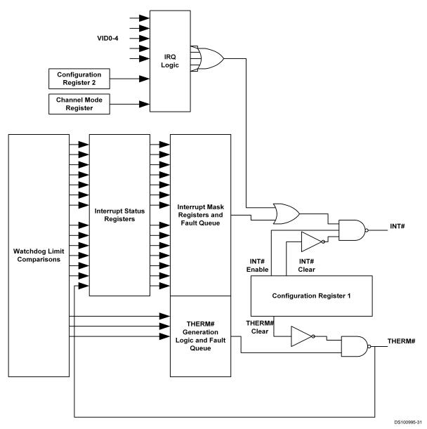
FIGURE 10. Interrupt Structure
