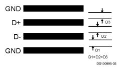
FIGURE 9. Recommended Diode Trace Layout
