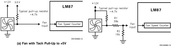
(a) Fan with Tach Pull-Up to +5V
