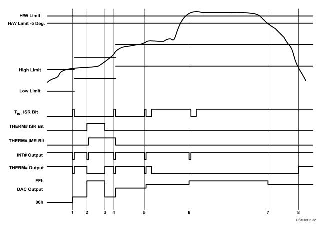
FIGURE 11. LM87 Interrupt Structure
