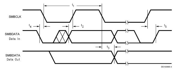
FIGURE 1. Serial Bus Timing Diagram
