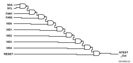
FIGURE 12. NAND Tree Test Structure
