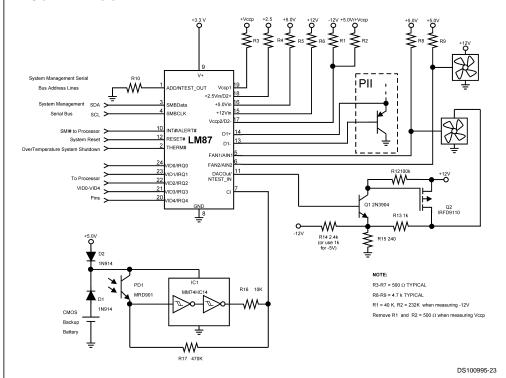
FIGURE 13. In this PC application the LM87 monitors temperature, fan speed for 2 fans, and 6 power supply voltages. It also monitors an optical chassis intrusion detector.
