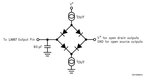
FIGURE 3. Digital Output Load Test Circuitry
