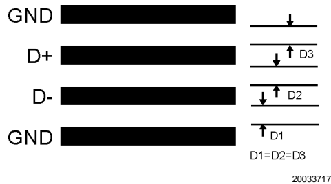
FIGURE 15. Ideal Diode Trace Layout
