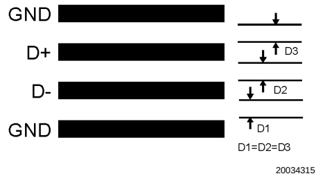
FIGURE 6. Recommended Diode Trace Layout
