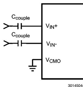
**FIGURE 12. Differential Analog Input Connection**
