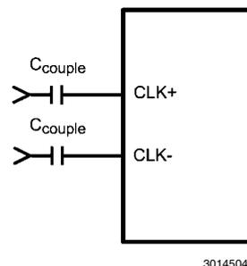
**FIGURE 15. Differential Sample Clock Connection**
