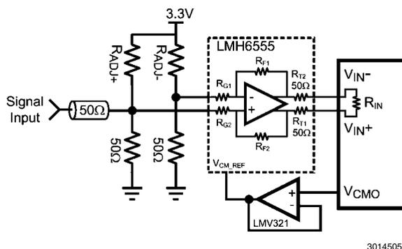
FIGURE 14. Example of Servoing the Analog Input with  $V_{CMO}$
