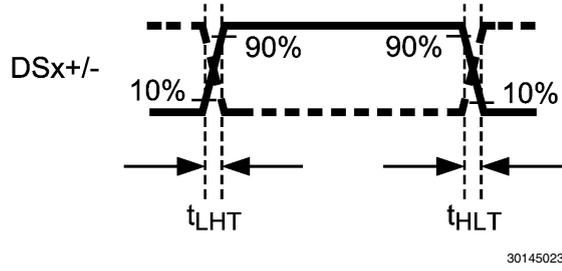
FIGURE 3. Output Data Timing
