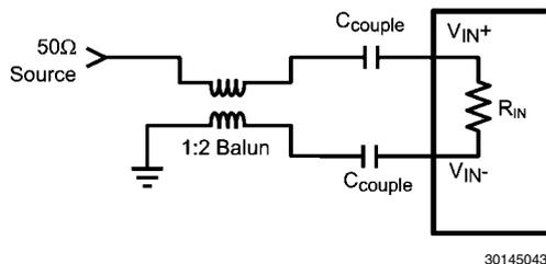
FIGURE 13. Single-Ended to Differential signal conversion with a balun
