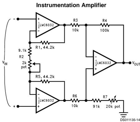
$$\frac{V_{OUT}}{V_{IN}} = \frac{R2 + 2R1}{R2} \times \frac{R4}{R3}$$
