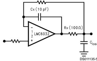
**FIGURE 3. Rx, Cx Improve Capacitive Load Tolerance**
