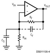
$C_S$  consists of the amplifier's input capacitance plus any stray capacitance from the circuit board and socket.  $C_F$  compensates for the pole caused by  $C_S$  and the feedback resistor.
