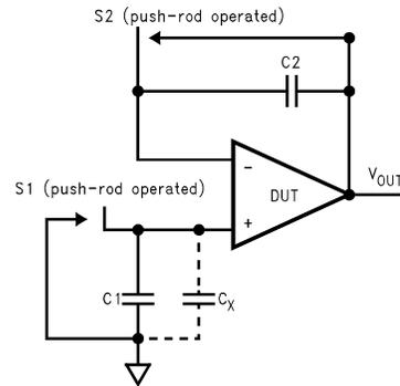
FIGURE 8. Simple Input Bias Current Test Circuit
