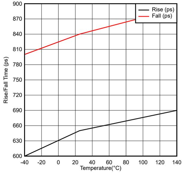
**Figure 5-5. Rise and Fall Time with 100pF Load**
