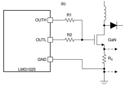
**Figure 7-3. Source Resistor Current Sense B Configuration**
