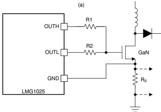
**Figure 7-2. Source Resistor Current Sense A Configuration**
