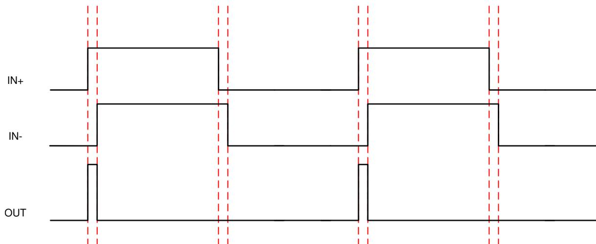
**Figure 7-5. Timing Diagram To Create Short Pulses**
