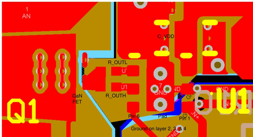
Figure 9-1. Typical LMG1025-Q1 Layout With Ball-Grid GaN FET
