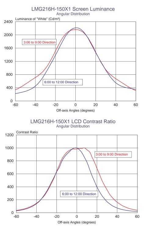
The "white" color displayed on the screen when the video signal is applied may have a slightly lower luminance. When the LCD is properly driven, the luminance of the "white" color displayed on the screen should be within 5% of the specified value.
