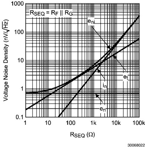
FIGURE 9. Voltage Noise Density vs. Source Resistance
