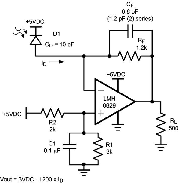
$V_{out} = 3VDC - 1200 \times I_D$
