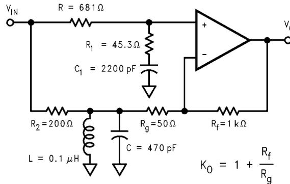
$$\frac{V_O}{V_{IN}} = K_0 \left( \frac{sC_1 R_1 + 1}{sC_1 (R_1 + R) + 1} - \left( \frac{R_f}{R_f + R_g} \right) \frac{sLR_g}{s^2 LCR_2 R_g + sL(R_2 + R_g) + R_2 R_g} \right)$$
