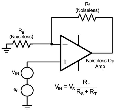
**FIGURE 7. Non-Inverting Amplifier Equivalent Noise Source Schematic**
