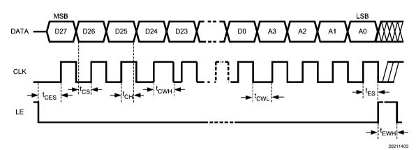
Data bits set on the DATA signal are clocked into a shift register, MSB first, on each rising edge of the CLK signal. On the rising edge of the LE signal, the data is sent from the shift register to the addressed register determined by the LSB bits. After the programming is complete the CLK, DATA, and LE signals should be returned to a low state.
