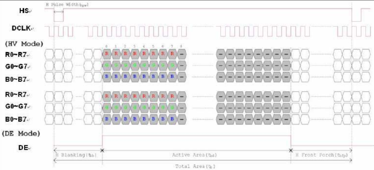
1 Horizontal input timing diagram.
