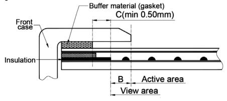
3. The front case side wall should keep space (e.g.  $0.2 \sim 0.3$ mm) from the touch panel.
