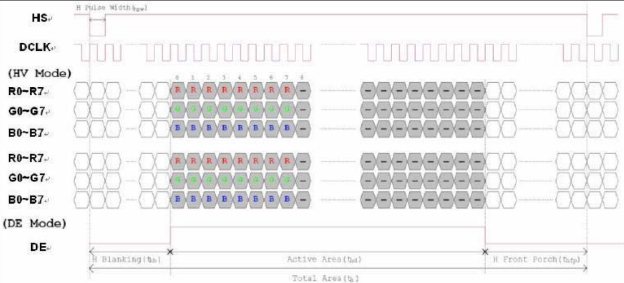
1 Horizontal input timing diagram.
