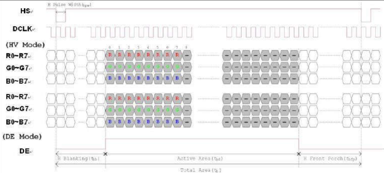
1 Horizontal input timing diagram.
