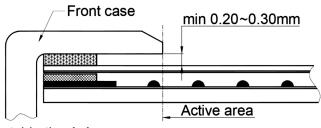
Outer case design should take care about the area outside the A.A. Those areas contain circuit wires which is having different thickness. Touching those areas could deform the ITO film. As a result case the ITO cold be damaged and shorten its lifetime. It is suggested to protect those areas with gasket (between the front case and the touch panel). The suggested figures are B≥0.50mm; C≥0.50mm₀
