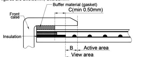
The front case side wall should keep space (e.g. 0.2 ~ 0.3mm) from the touch panel.
