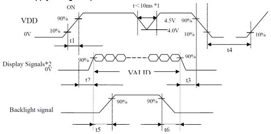
**Timing:** 0.47ms<t1 <10ms; 0.5 ms<t2 <50ms; 0ms<t3 <50ms; t4 >1000ms; t5 >200ms; t6 >200ms;
