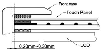
In general design, touch panel V.A. should be bigger than the LCD V.A. and touch panel A.A. should be bigger than the LCD A.A.
