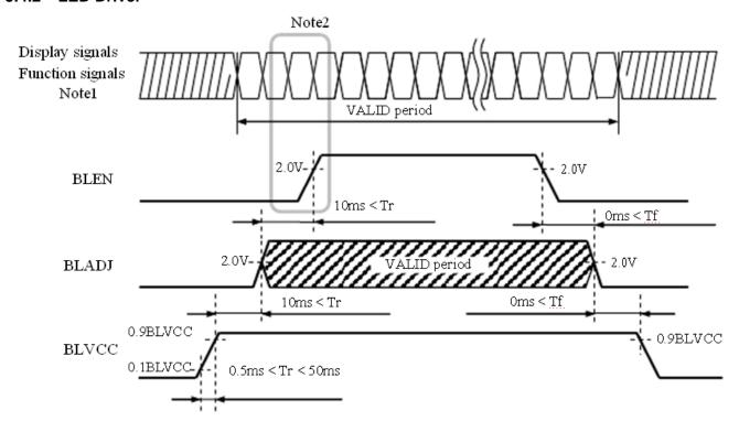
Note1: These are the display and function signals for LCD panel signal processing board.
