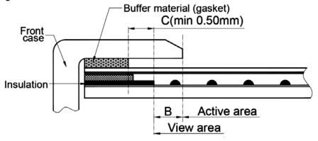
3. The front case side wall should keep space (e.g. 0.2 ~ 0.3mm) from the touch panel.
