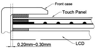
4. In general design, touch panel V.A. should be bigger than the LCD V.A. and touch panel A.A. should be bigger than the LCD A.A.
